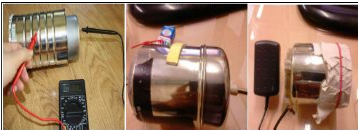
Figure 2: Instrumentation developed for the Ionization chamber and Radon Collector
